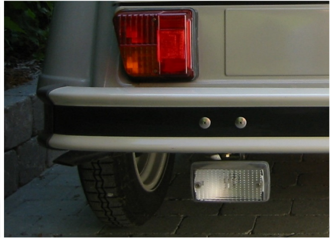
Reversing lamp from PR 3493 (June 2, 1986). The switch for this lamp is integrated in the rear gearbox cover. This rear gearbox cover and switch was also fitted on Méhari USA versions around 1970.
