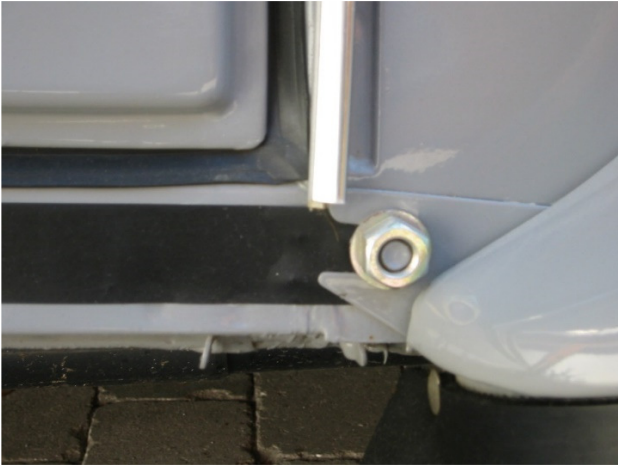
Protective chromed plastic trim AZ 851-125a on rain gutter. See also note under Charleston model year 1985. cover.
