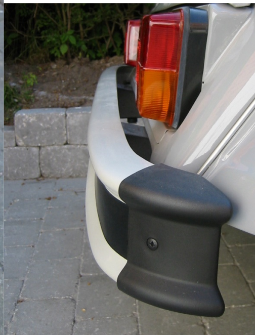
Protectors on front bumper corners and on overriders, and protectors on rear bumper corners. From November 1980 or from PR 1515 (Jan. 1, 1981) - the sources are ambiguous.
