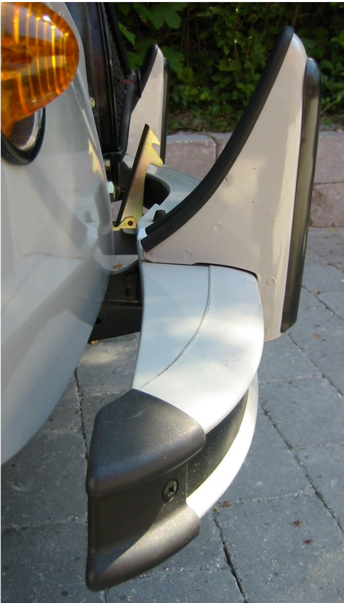
Protectors on front bumper corners and on overriders, and protectors on rear bumper corners. From November 1980 or from PR 1515 (Jan. 1, 1981) - the sources are ambiguous.
