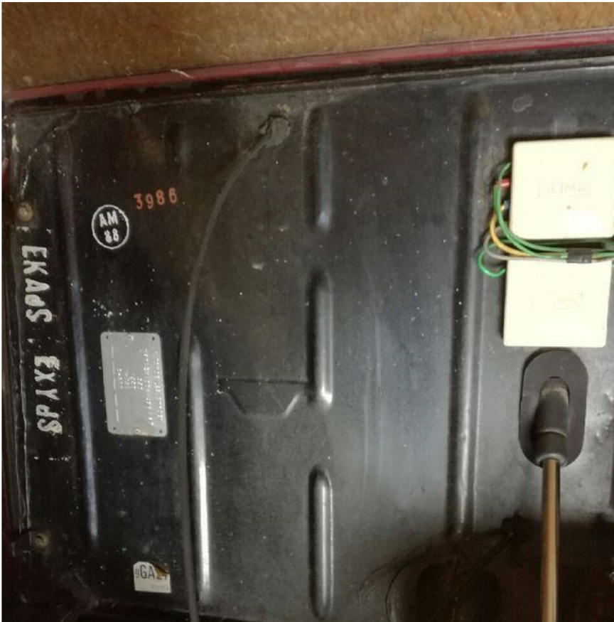
Firewall on a Levallois-built model year 1988 Rouge Delage/Noir Charleston: Color codes "EKA" = Rouge Delage and "EXY" = Noir. "AM 88" meaning Année Modèle (model year) 1988. The AM stamp is not present on all markets. "3986" is the PR-number = manufacturing date October 8, 1987.
