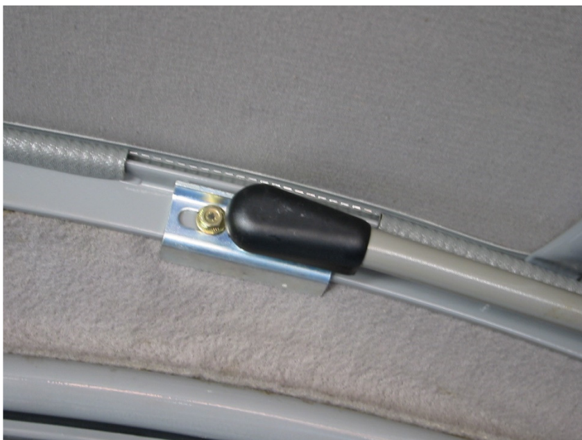
Black protector on sunroof bracket hinge. Light gray protector along the top edge of the bodyshell. The latter from PR 2426 (July 1, 1983)
