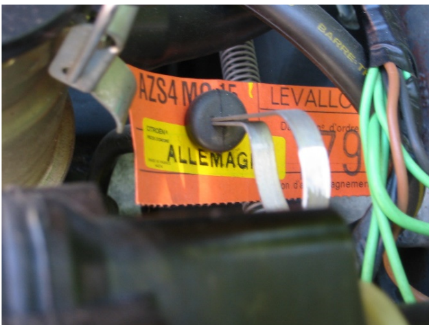
West Germany engine labels on A 06/664 engine. "Taux reduit 7-9" = "Reduced compression ratio" 7.9:1. From PR 3157 (July 1, 1985).
