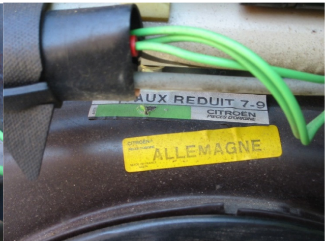
West Germany engine labels on A 06/664 engine. "Taux reduit 7-9" = "Reduced compression ratio" 7.9:1. From PR 3157 (July 1, 1985).
